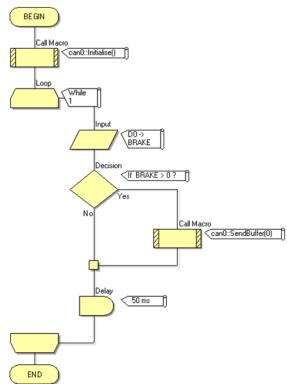
Figure 7.1 Send signal flowchart
