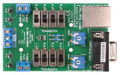
conditions: short circuit to 5V, short circuit to ground, open circuit and partial open circuit. The potentiometers RV1 and RV2 allow you to vary the partial open circuit resistance. The circuit of the CAN faults board is available in the technical datasheet of the CAN faults board.
