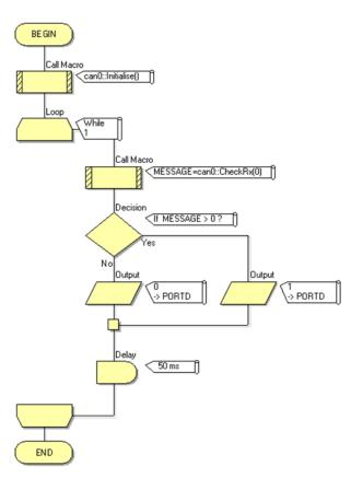
Figure 7.2Receive signal flowchart
