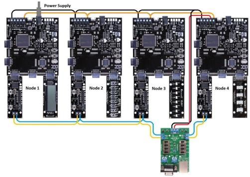
Figure 6.1 CAN System – System overview
