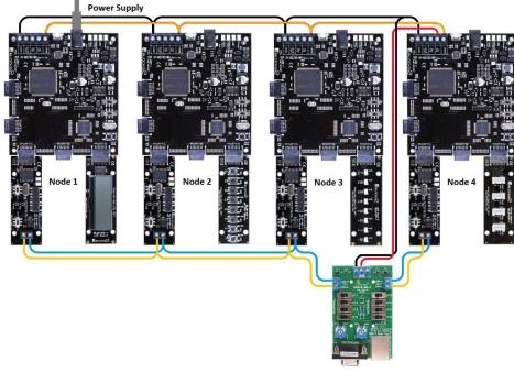
Figure 3.3 CAN system – wiring of the power connections
