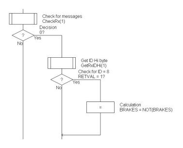
Figure 14.1 Code fragment showing how to retrieve the message ID
