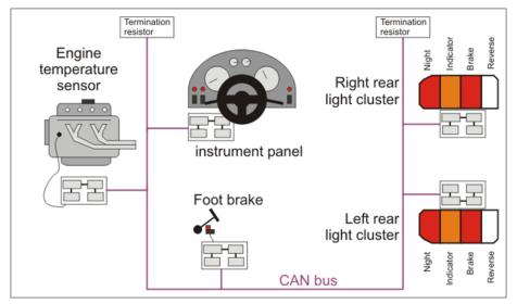
Figure 2.1 Typical automotive CAN bus arrangement
