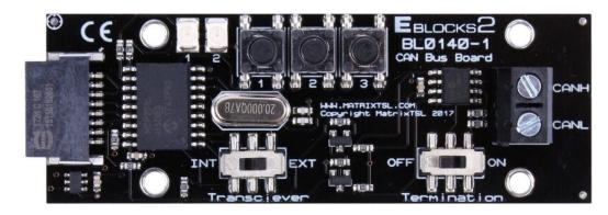
Figure 3.2 The E-blocks2 BL0140 CAN board
